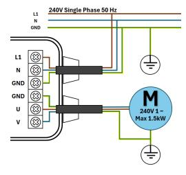
The terminal block inside the controller is clearly labelled. Incorrect wiring will destroy the electronic circuit board.
